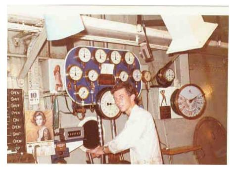
trolling the engine directly with big levers and valves. It was loud, hot and relatively primitive, but had the great advantage of being reliable. Ships of that vintage did not have much in the way of automation, so it was all "handamatic".
