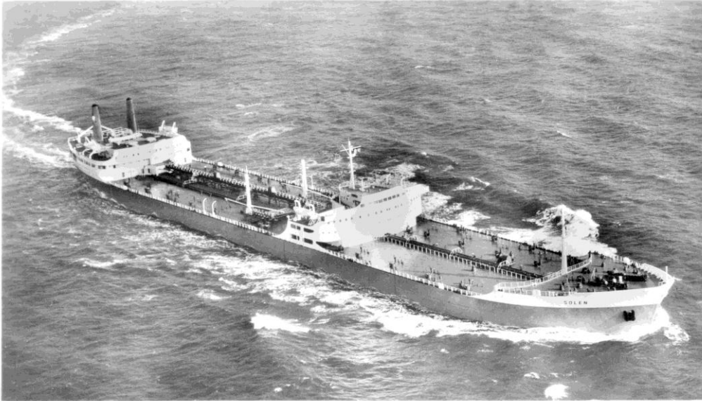
SHELL TANKER s.s. "SOLEN" 67,848 D.W. TONS. 16,250 SHP 77000
