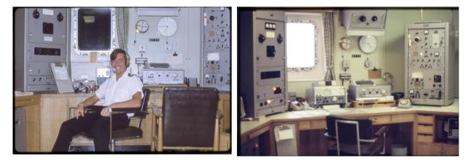
The radio equipment was relatively good, consisting of the Marconi Crusader 1.5
